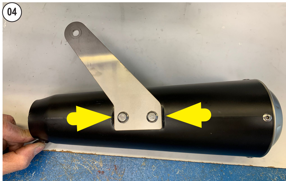
INSTALL THE BRACKET ON LEOVINCE MUFFLER - REMEMBER THE GASKET
