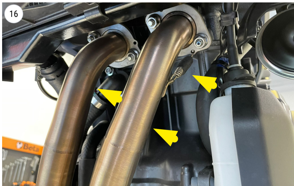
fit the primary pipes
